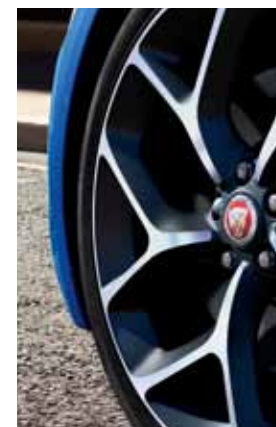
20" 10-Spoke 'Style 1014' Satin Grey & Diamond Turned Finish O29UG Banden vóór / achter: 235/35 R20 92Y / 265/30 R20 92Y zomerbanden
